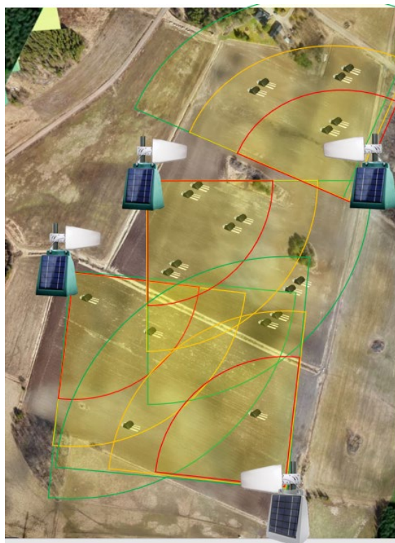
Figure 3. Placement of 20 wireless soil sensors and data repeaters (SoilScout) in the different soil zones of the experimental fields.
