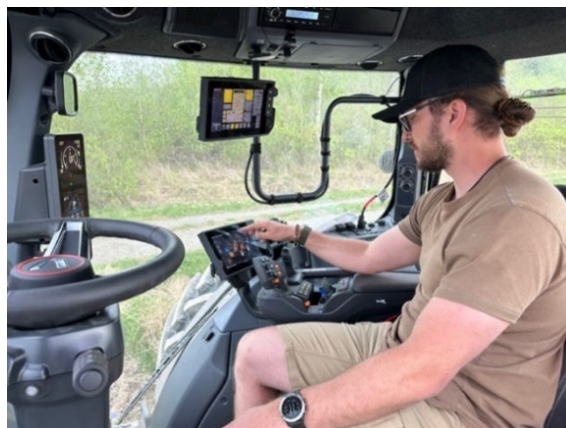
Figure 2. The tractor (Valtra N175D) with autosteer and automated headland turning functionalities.
