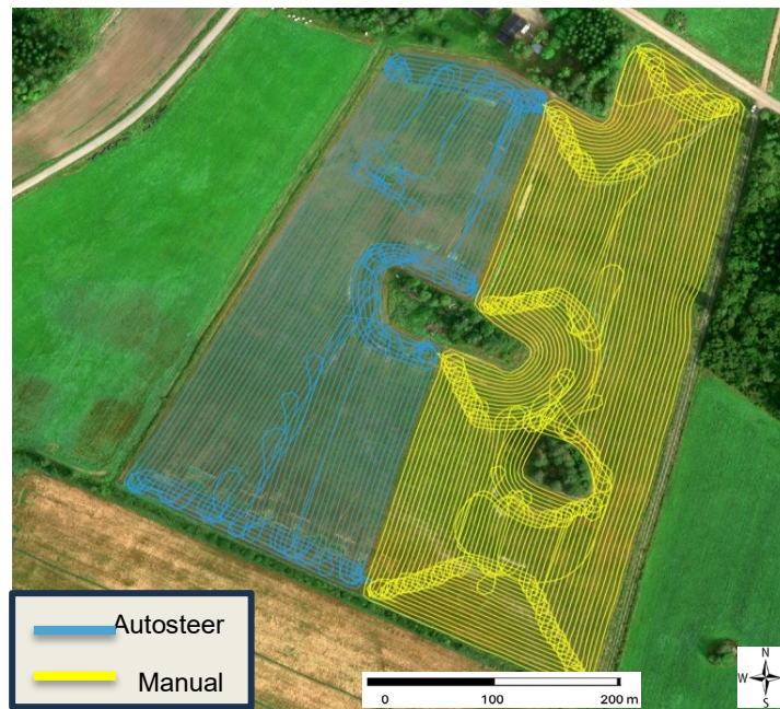
Figure 6. Driving patterns during seeding in 2022 (as visualized in QGIS). Manual operation (right) and autosteer (left).
