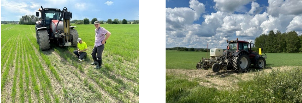
Figure 4. Soil scanning (Veris) and deep soil sampling (Wintex) of the test fields.
