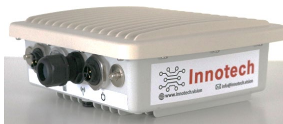
Figure 2. The data processing and communication unit of the WD system before deployment.
