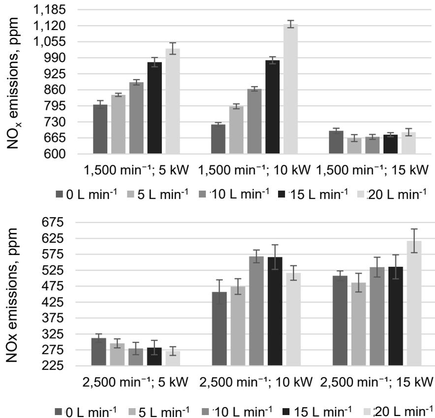
**Figure 7.** Variation of NO<sub>x</sub> emissions under different load modes and hydrogen flow rates.
