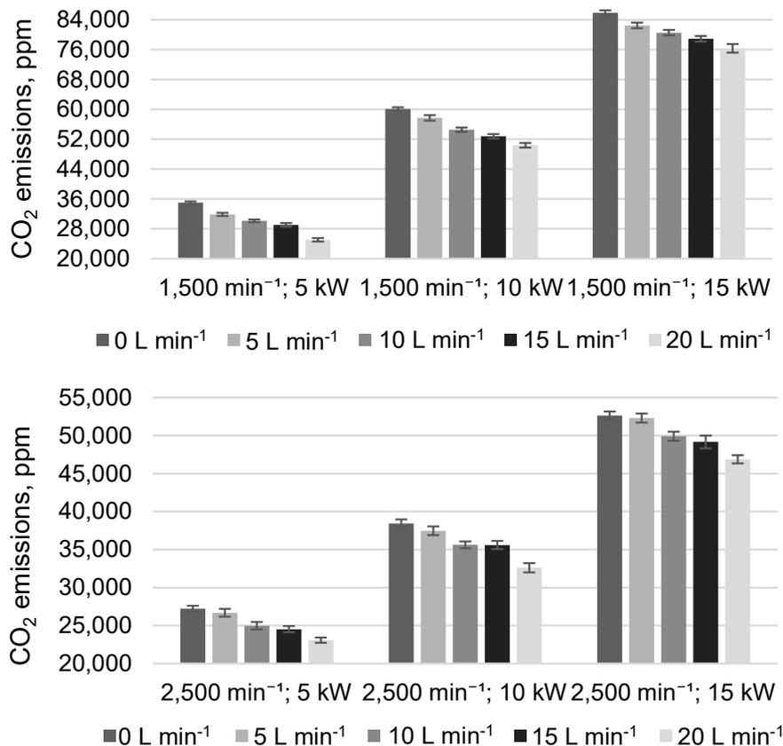
**Figure 4.** Variation of CO<sub>2</sub> under different load modes and hydrogen flow rates.
