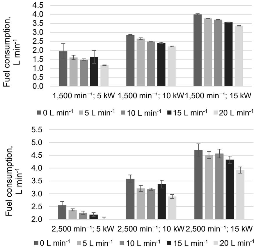
**Figure 3.** Variation of fuel consumption under different load modes and hydrogen flow rates.
