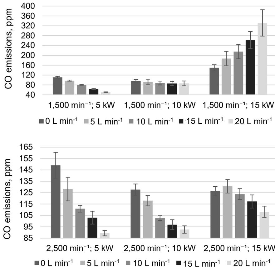
**Figure 5.** Variation of CO emissions under different load modes and hydrogen flow rates.
