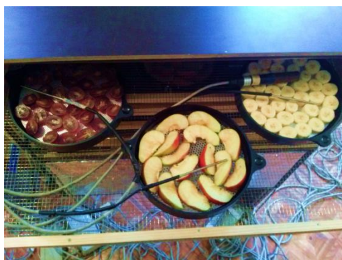
Figure 2. Samples at the beginning of the drying experiment.
