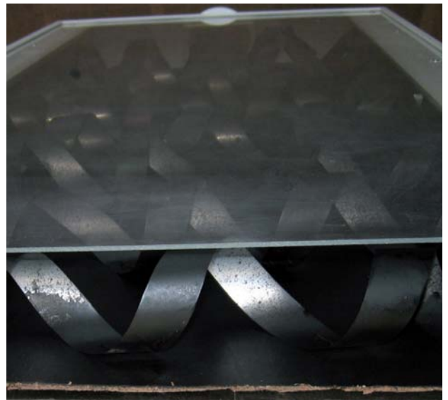
Fig. 6. Air heating solar collector with absorber black colored slices of beer cans.
