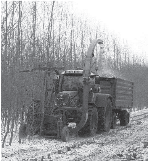
Figure 4. ATB mower-chipper at harvest of poplar (2013).
