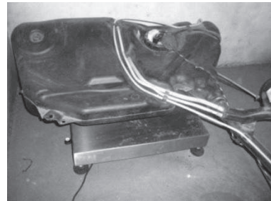
Figure 10. Position of the tank on the platform scale.
