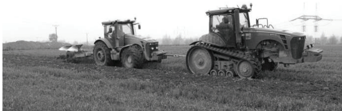
Figure 1. The measuring set during the measurement of tensile force using the tensile dynamometer LUKAS type S-38.
