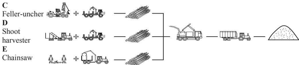
**Figure 4.** Cut-and-storage harvest of wood chips from SRC.
