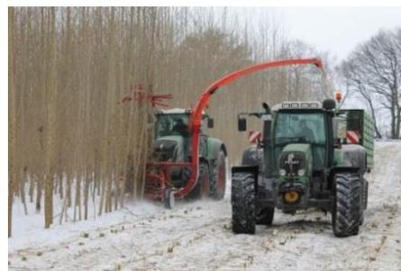
**Figure 3.** ATB mower-chipper.
