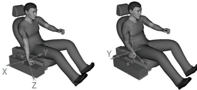
Figure 2. Position of the driver when gripping the handle of the mechanical handbrake with a classic design
