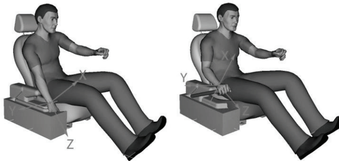
Figure 4. Position of the driver whilst gripping the handle of the handbrake with the structural design solution in both extreme positions.
