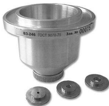
**Figure 1.** The viscometer VZ–246.
