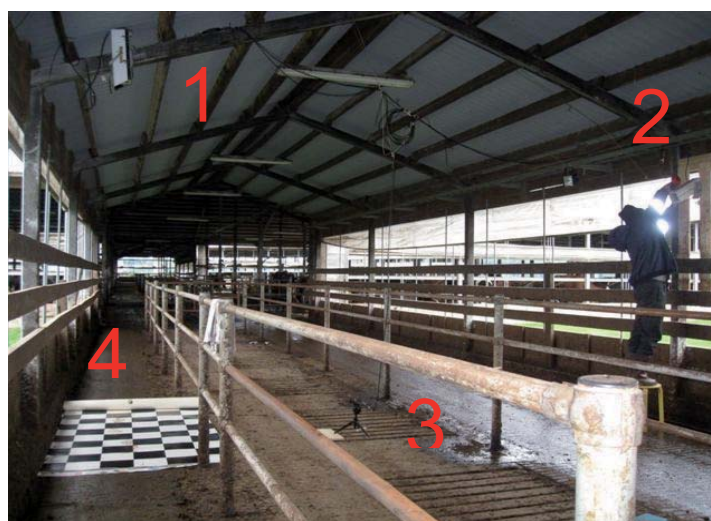
Fig. 5. Installation of video-system in the cowshed: 1 – top camera; 2 – side camera; 3 – hoof camera; 4 – calibration mat.
