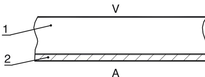
**Figure 2.** Scheme of modelling briquette. 1 – substrate briquette; 2 – board; V – surface of heat exchange with room air (briquette top); A – surface of heat exchange with room air through board (briquette bottom).
