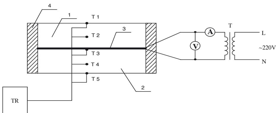
**Figure 1.** Scheme of measuring nonsteady temperature regime in substrate briquettes: 1, 2 – substrate briquettes, 3 – flat thin heater of constant power, 4 – thermal insulation, V, A – measuring devices, T – transformer,  $T_1 - T_5$  – temperature sensors, TR – recording device.
