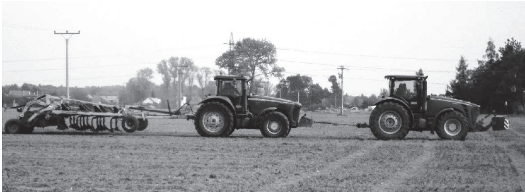
Figure 1. Measuring set. From right: pulling tractor John Deere 8345R, measuring instrument, pulled tractor John Deere 8220 for lifting and lowering of the cultivator, cultivator Ecoland EO 4000.
