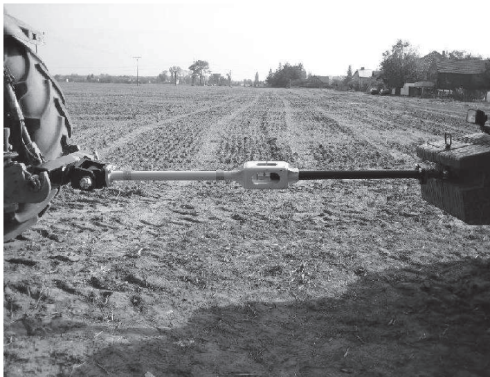
Figure 2. Measuring equipment between the pair of tractors.
