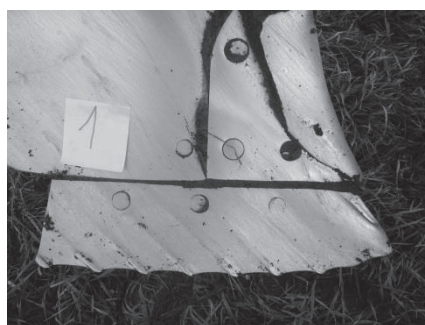
Figure 11. Wear of ploughshare (M1) after ploughing 18 ha.
