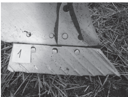
Figure 8. Wear of ploughshare (M1) after ploughing 12 ha.
