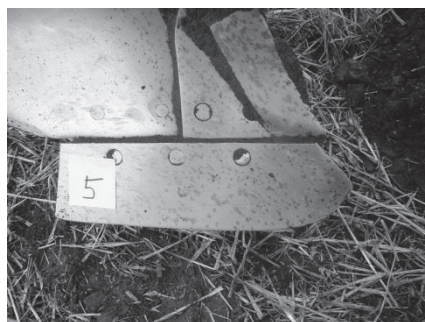
Figure 9. Wear of ploughshare (etalon) after ploughing 12 ha.
