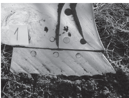
Figure 10. Wear of ploughshare (M1) after ploughing 14 ha.
