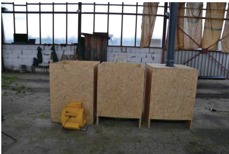
Figure 1. Storage container with active ventilation (on the left), with passive ventilation (on the right), and check container (in the middle).
