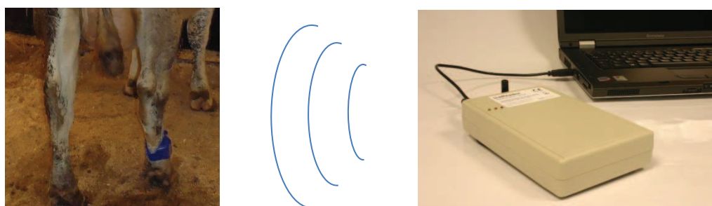
Figure 1. Eksperiment layout: IceTag sensor is attached to cow's right hind leg (left) and reading device (right) is communicating with it by radiolink.
