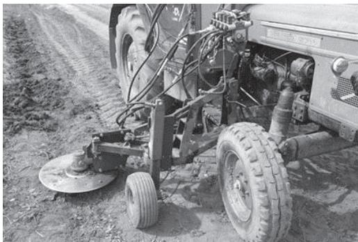
**Figure 1.** Experimental model of mechanical pruner placed on tractor.
