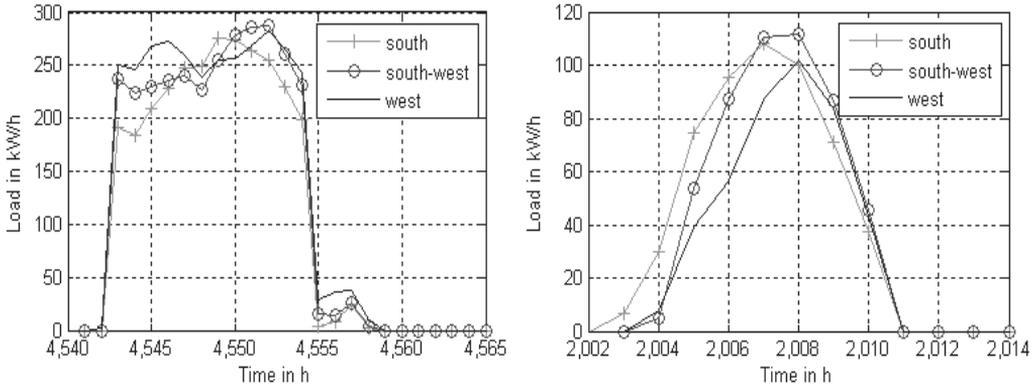
**Figure 4.** Hourly values of the cooling load in an average summer and spring day.
