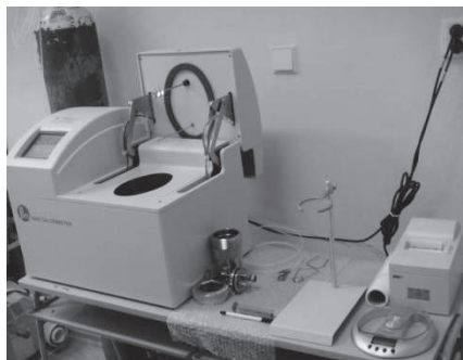
Figure 6. Testing instrument – PARR 6200 Calorimeter.
