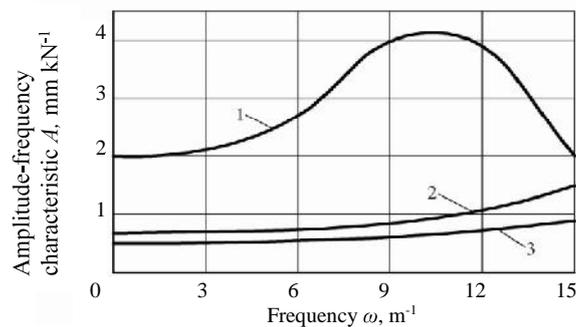
**Figure 13.** Amplitude frequency response characteristic of vertical oscillations of plough, when it responds to variation of its own tractive resistance at different coefficients of stiffness  $C_{TP}$  of tyre on its ground support wheel: 1 –  $100 \text{ kN m}^{-1}$ ; 2 –  $150 \text{ kN m}^{-1}$ ; 3 –  $200 \text{ kN m}^{-1}$ .
