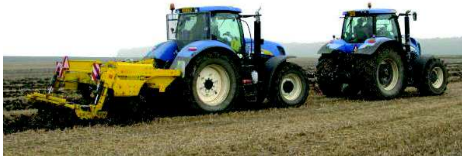
Figure 1. Photo of draft measurement of chisel plough Strom Terraland TN 3000 at Sloveč in autumn 2014.
