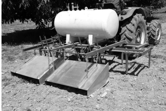
Figure 1. The weed flamer developed in this study.
