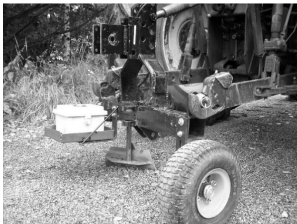
Figure 1. IRMA 7 D sensor mounted to a three point hitch frame.
