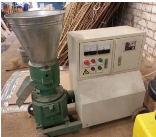
Figure 1. Small capacity granulator with a horizontal granulator matrix.
