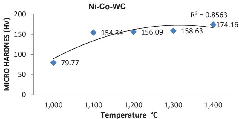
**Figure 2.** The micro hardness tests results from sintered specimens treated at various temperatures.
