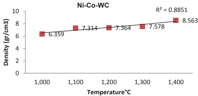
**Figure 1.** The density change with respect to sintering temperature.
