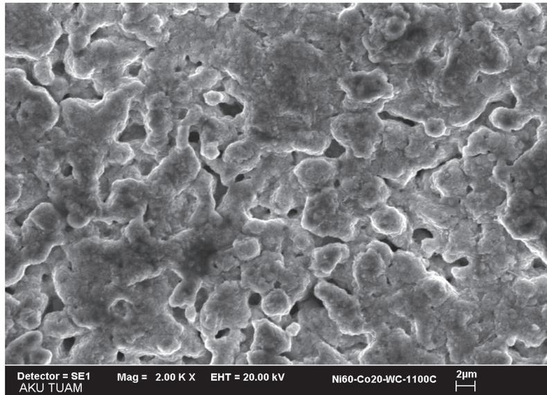
**Figure 7.** SEM view of (Ni-Co-WC) composite 1,100 °C.
