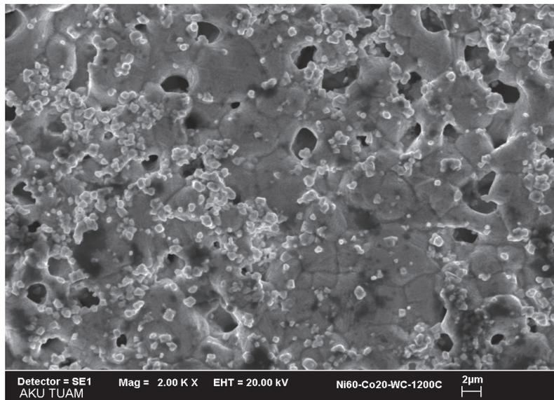
**Figure 6.** SEM view of (Ni-Co-WC) composite 1,200 °C.
