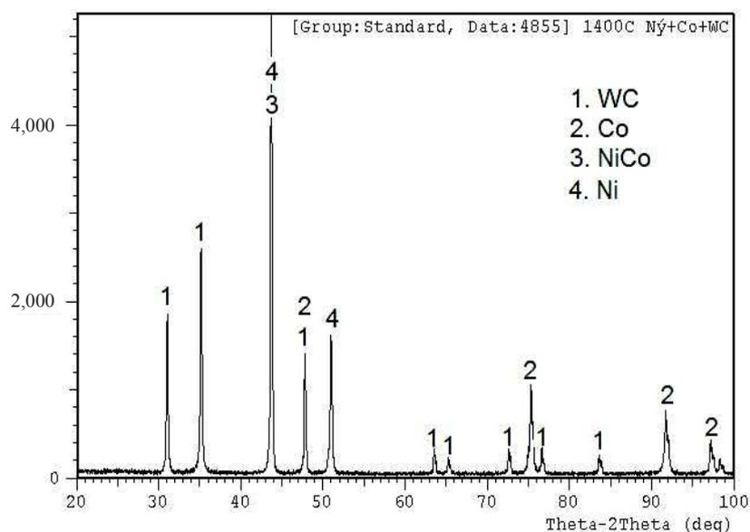
**Figure 9.** The XRD analysis (Ni-Co-WC) composite Sintered in tube furnace at 1,400 °C.
