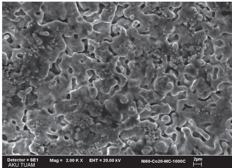
**Figure 8.** SEM view of (Ni-Co-WC) composite 1,000 °C.
