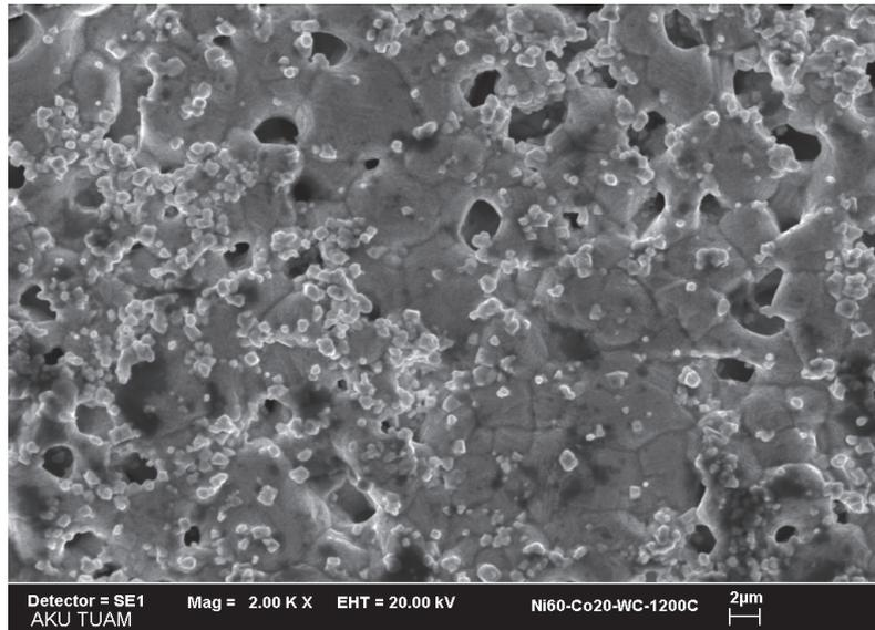
**Figure 6.** SEM view of (Ni-Co-WC) composite 1,200 °C.
