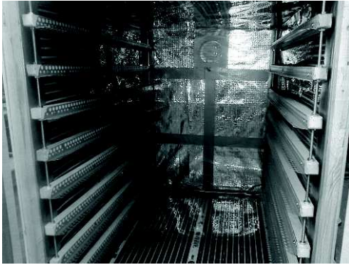
Figure 1. IR dryer shelving system.
