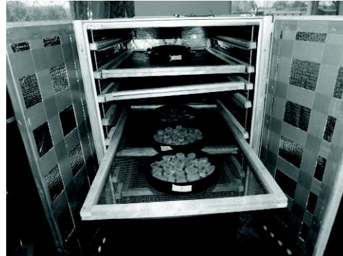
Figure 2. IR dryer with carrot in practice.
