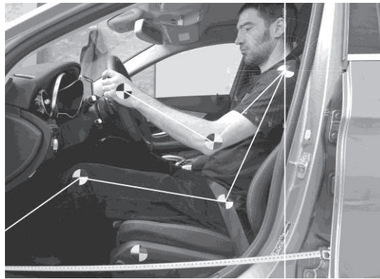
Figure 3. Tested subject, photographed in measurement position with designated flowlines of joints.
