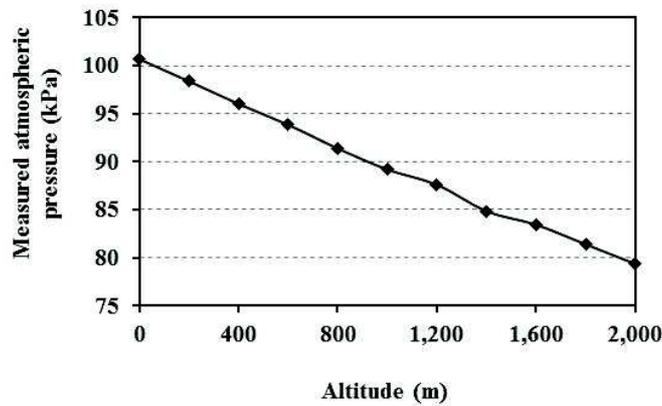
**Figure 4.** Measured atmospheric pressure as affected by the altitude.
