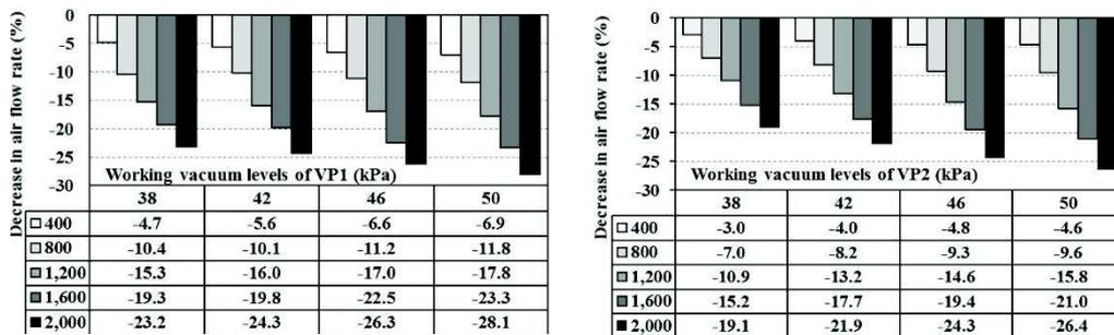
**Figure 8.** Air flow rate losses of the vacuum pumps at different altitudes and working pressures.
