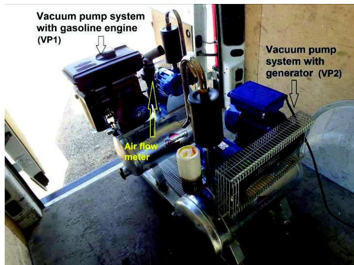
**Figure 1.** VP1 and VP2 driven by gasoline engine and generator, respectively.
