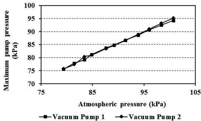
**Figure 6.** Maximum pressure and true air pressure relations of VP1 and VP2.
