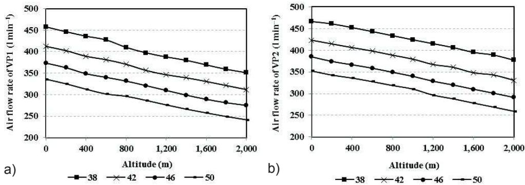
**Figure 7.** The effect of altitude on air flow rate of vacuum pumps at pressure range of 38–50 kPa for VP1 and VP2.
