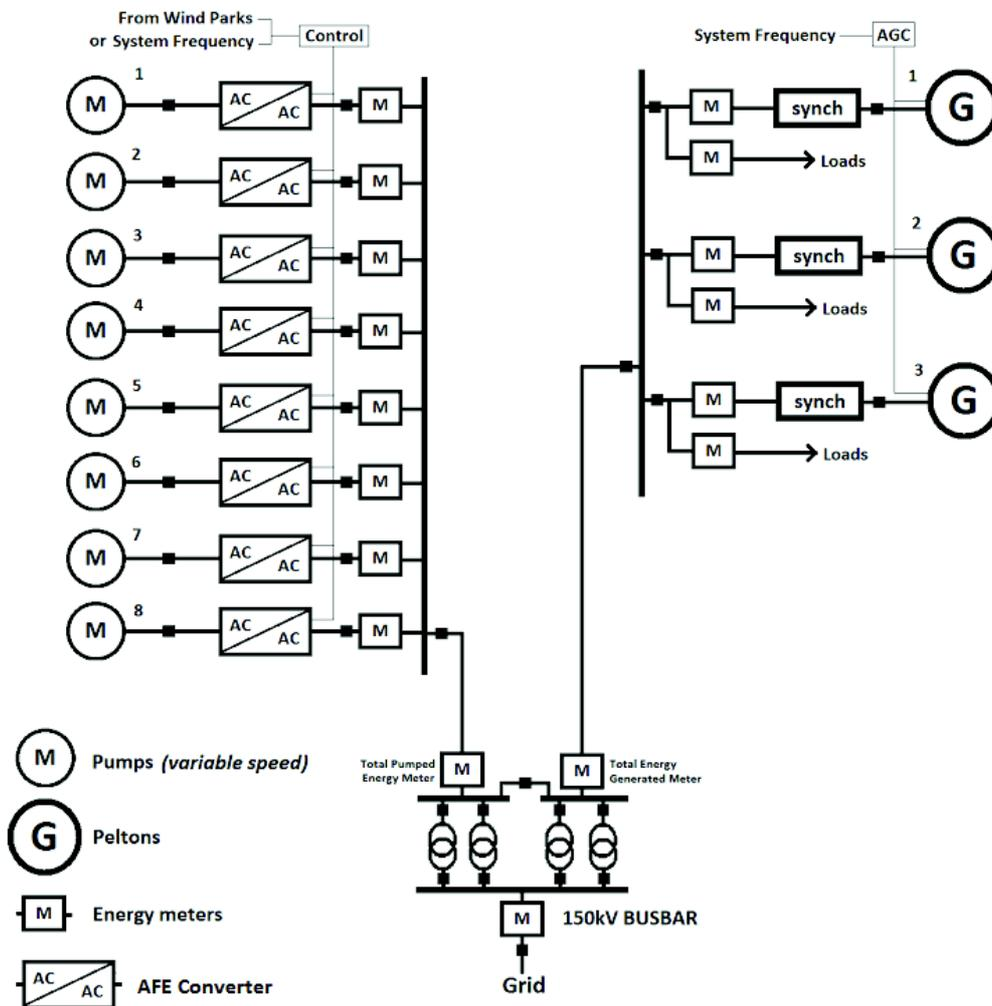
Figure 2. Single line diagram of the examined project.
