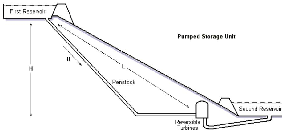
**Figure 1.** Components and structure of pump hydro storage system.
