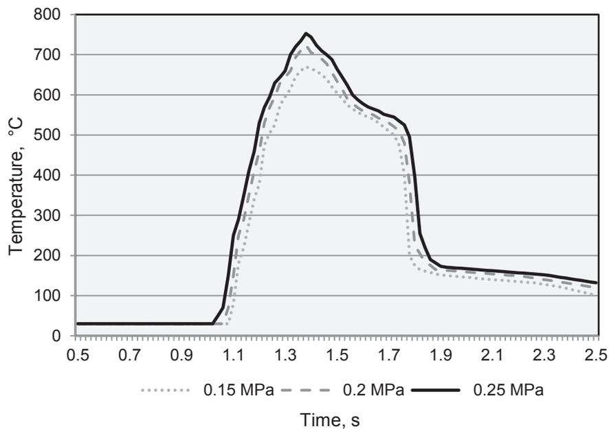
**Figure 4.** Measurement of thermal characteristics of flame weeder Reinert – DA211at speed of 2 km h<sup>-1</sup>.
