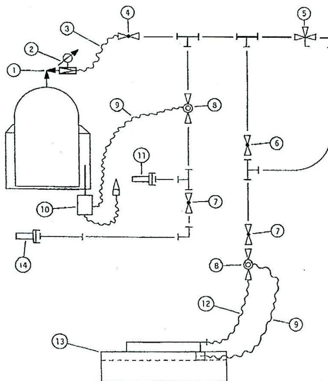
**Figure 2.** Gas flow scheme Reinert – DA211: 1 – gas bottle; 2 – pressure regulator; 3 – connecting hoses; 4 – throttle valve; 5 – starter; 6 – quick shutter; 7 – shut-off valve; 8 – safety valve; 9 – thermal fuse; 10 – thermal sensor; 11 – heating bottles; 12 – supply hoses; 13 – burner; 14 – ignition burner.
