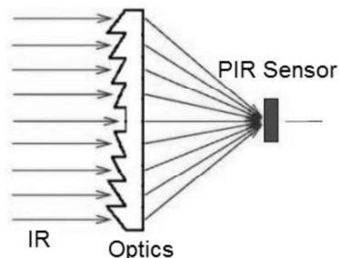
**Figure 1.** Schematic showing the PIR sensor function.
