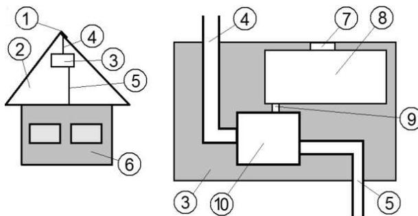
**Figure 4.** Distribution system: 1 – Sprayers; 2 – Roof; 3 – Tank; 4 – Mixed piping; 5 – Water supply system; 6 – Greenhouse; 7 – refilling opening; 8 – Integrated refilling tank; 9 – Dispenser; 10 – Mixing chamber.
