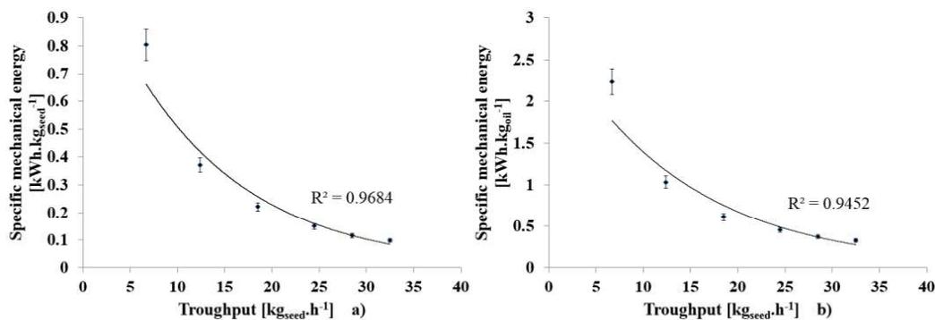
**Figure 3.** Dependence between seed material throughput and mechanical energy for a) pressing one kilogram of rapeseeds; b) obtaining one kilogram of oil.
