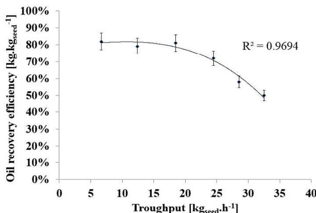
**Figure 4.** The effect of seed material throughput on oil obtained ratio.
