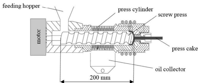
**Figure 1.** Scheme of mechanical screw press for oil extraction (Karaj & Müller, 2011).
