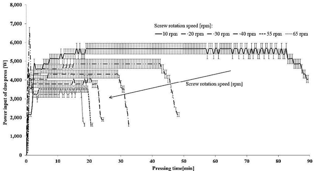
**Figure 2.** Effect of screw rotation speed on electric power input of duo press and pressing time for 10 kg of rapeseeds.
