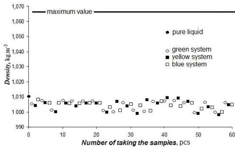
**Figure 4.** The trend of density at 25 °C.
