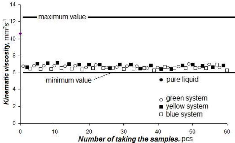
**Figure 3.** The trend of kinematic viscosity at 40 °C.
