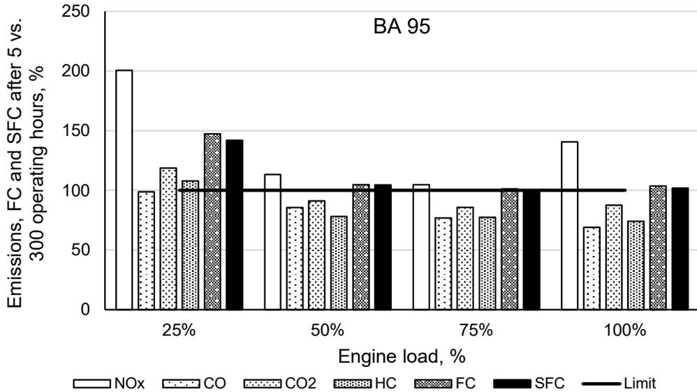
**Figure 2.** Percentage comparison of emissions production and fuel consumption of the generator operating on petrol (BA 95) after 5 operating hours (100%) and 300 operating hours. (FC – fuel consumption, SFC – specific fuel consumption)
