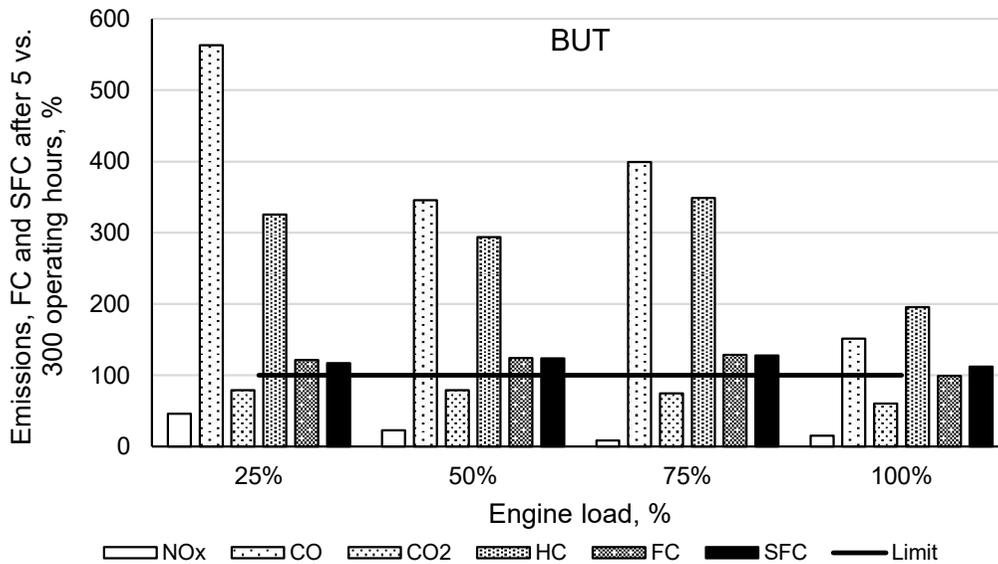
**Figure 3.** Percentage comparison of emissions production and fuel consumption of the generator operating on n-butanol (BUT) after 5 operating hours (100%) and 300 operating hours. (FC – fuel consumption, SFC – specific fuel consumption).
