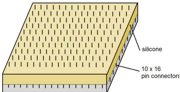
**Figure 2.** Pin connector matrix.
