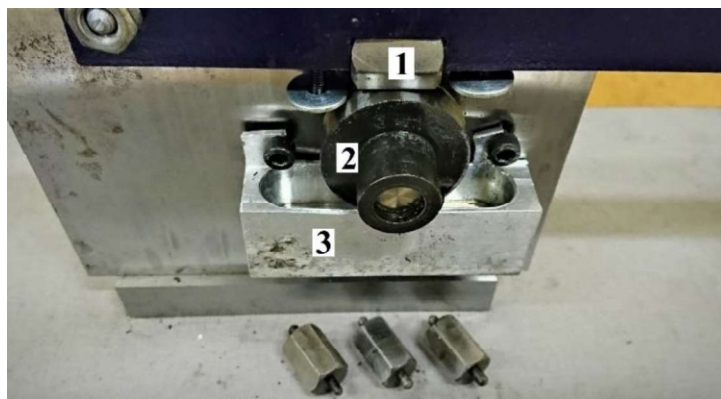
Figure 4. Side view of sliding friction test bench with friction blocks used in the tests: 1 – friction block; 2 – steel disc; 3 – oil reservoir.
