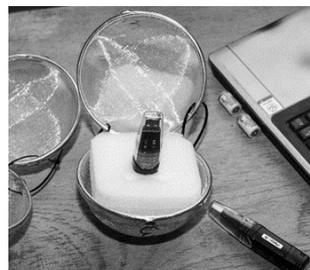
**Figure 2.** Placing a datalogger into a protective sieve.
