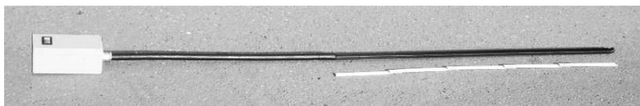
**Figure 7.** Realized frost depth indicator.
