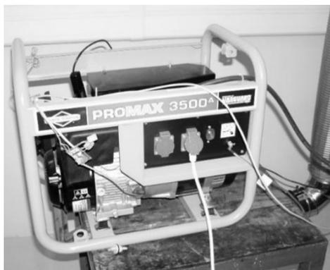
**Figure 1.** Mobile generator ProMax 3500A powered by small Briggs and Stratton engine type Vanguard 6.5HP.
