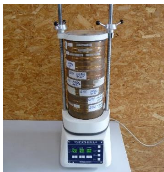
Figure 4. The test sieve shaker (sieve analyzation).
