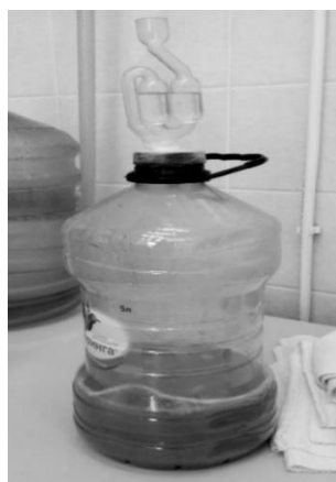
Figure 3. Hand-made fermenter for fermentation of wort pitched with angkak .
