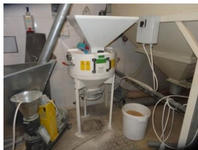
Figure 3. Hammer mill Taurus.
