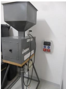
Figure 1. Two roller mill VKM 130/150.
