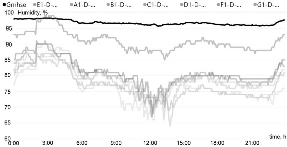
**Figure 8.** uMOL system D level relative humidity readings per poles A-H comparing to humidity deficit values (bold).
