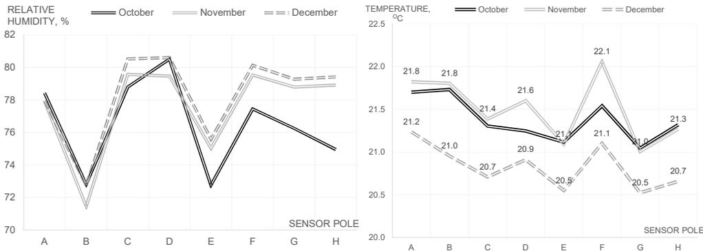
**Figure 9.** uMOL system monthly average relative humidity (left) and temperature (right) readings per sensor poles A-H.
