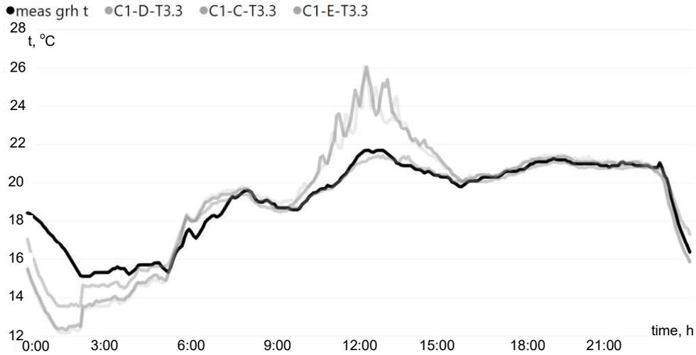
**Figure 6.** uMOL system and greenhouse temperature data comparison using only levels C,D,E (plant area).
