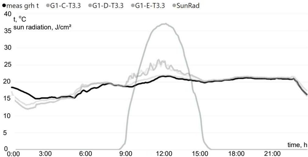
**Figure 7.** uMOL system G pole C,D,E sensor level, greenhouse temperatures (M=1:1) and sun radiation readings (M=1:20).
