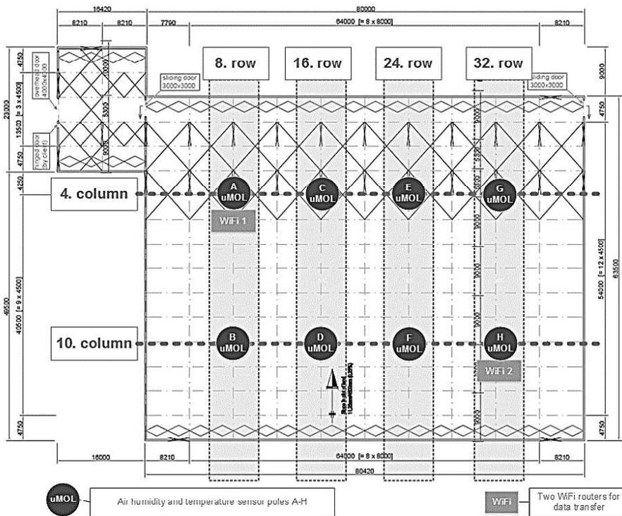
**Figure 1.** Typical industrial greenhouse layout and uMOL sensor pole A–H placement.
