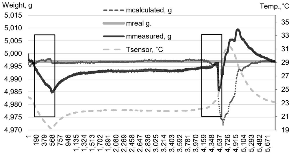
**Figure 2.** LSM reading stability experiment (impact of temperature test result).
