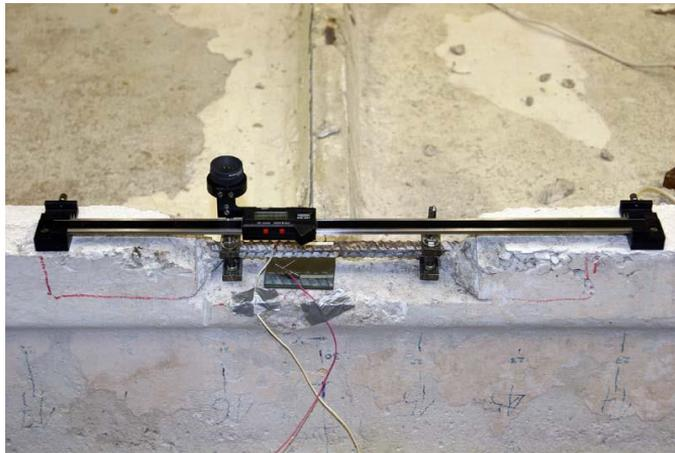
**Figure 6.** Pre-cleaned and pre-prepared PSB, with strain gauges and dummy gauge on the steel plate. Attached Helios Preisser Digi-Met 0 273 7 Digital Caliber 450 mm had insufficient accuracy (0.01 mm) and was applied only for approximate evaluation of longitudinal change of length of PSB.
