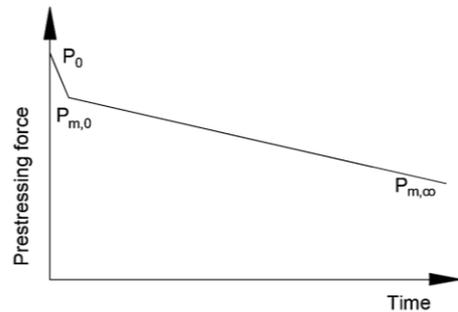
**Figure 2.** Principle of losses in prestressing force ( $P_0$ ) in time.
