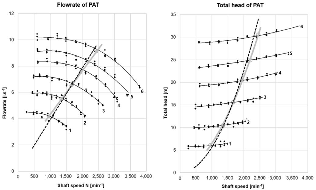
**Figure 5.** Predictive calculations of flowrate and total head versus reality.
