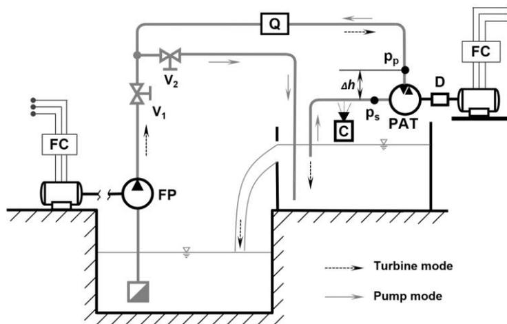
**Figure 3.** Hydraulic circuit scheme for testing turbines/pumps. Q – flowmeter, FP – feed pump; PAT – tested pump as turbine;  $V_1$ ,  $V_2$  – control valves; D – dynamometer; FC – frequency inverter; C – camcoder.
