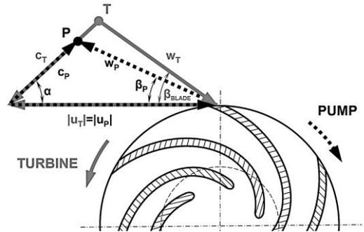
**Figure 1.** Kinematic conditions during pump and turbine operation.
