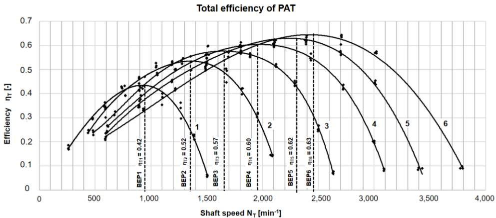
**Figure 4.** Courses of efficiency in modes 1 to 6 highlighting the optimum (BEP).
