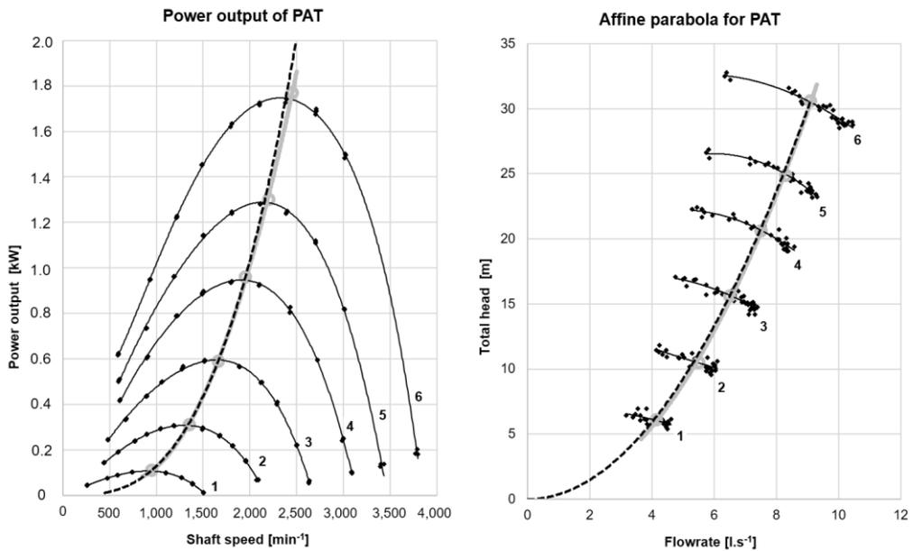
**Figure 6.** Predictive calculations of power output and affine parabola versus reality.
