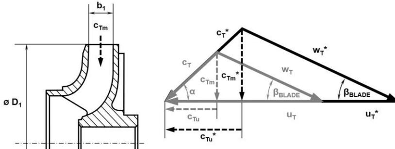
**Figure 2.** The change of kinematic conditions during turbine operation.
