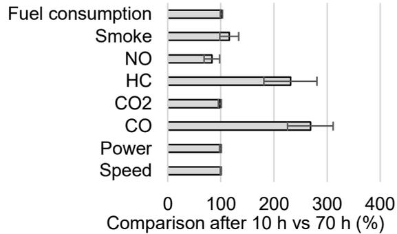
**Figure 4.** Change in emissions and fuel consumption in percent - 10 vs 70 h (diesel).
