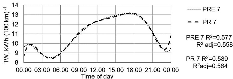
**Figure 2.** Car traction energy consumption regression lines on the test streets in the direction of the traffic lights green wave; PRE 7 – 7th order polynomial regression line with equalised endpoints, PR 7 – without equalised endpoints.
