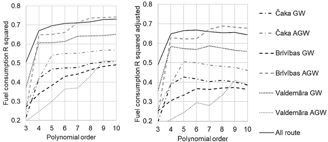
**Figure 5.** R squared and R squared adjusted values for fuel consumption 3rd to 10th order polynomial regression lines on test streets; GW – in the direction of green wave; AGW – in the direction against the green wave.
