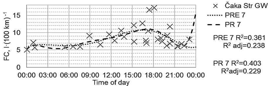
**Figure 3.** Car fuel consumption regression lines in the direction of the traffic lights green wave; PRE 7 – 7th order polynomial regression line with equalised endpoints; PR 7 – without equalised endpoints.
