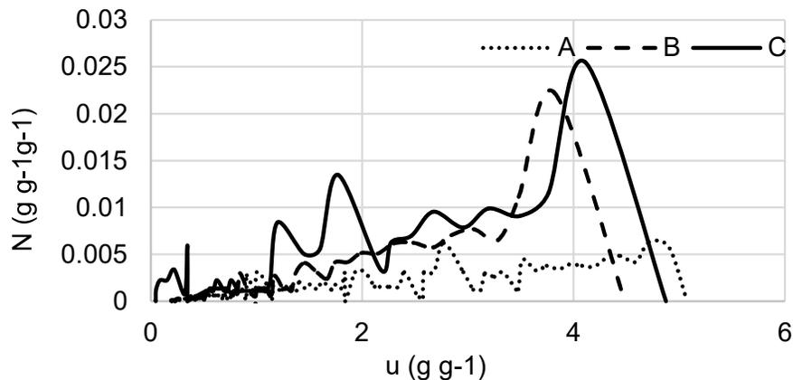
**Figure 5.** Drying rate  $N$  ( $\text{g g}^{-1}\text{min}^{-1}$ ) of 3 alfalfa samples as a function of water content  $u$  ( $\text{g g}^{-1}$ ) during the drying process.
