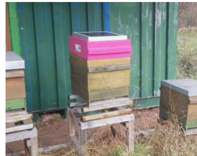
Figure 4. Bee hive with monitoring system prototype at the test site Witzenhausen of the University of Kassel.
