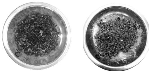
**Figure 1.** Digestate as a raw material without binder (left) and with addition of calcium carbonate (right).
