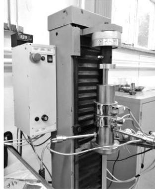
**Figure 2.** Testing stand for agglomeration process.
