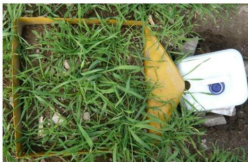
**Figure 2.** Microplot with a plastic container for measurement.
