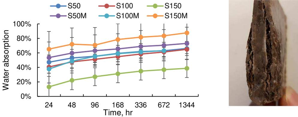
**Figure 8.** Water absorption of unmodified/modified HFRP composites with varying length of hemp fibres (Alao, 2018).
